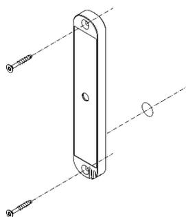
Now screw the device on the wall using the two countersunk screws provided.
