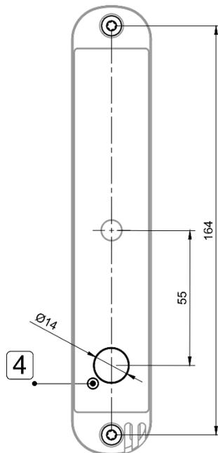
Mount the display in the area of the benches and keep a distance of at least 30 cm between the cabin ceiling and the upper edge of the device. Keep a minimum distance of 1 meter from the heater.
